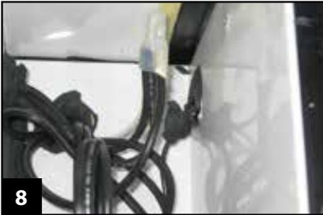
**STEP 13** - Disconnect power supply wires to thermometer on inside of cooler. (See image 8)
