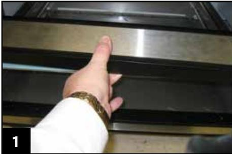
**STEP 4** - Remove the (4) Phillips screws holding the back assembly to the cabinet. (See image 2).
