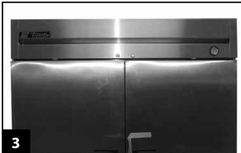
**STEP 3** - Remove the top, side, and bottom Phillips screw to the louver panel. (See image 3).
