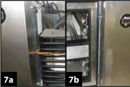
**STEP 11** - Remove (2) 1/4" screws on right-hand side of thermometer panel. (See image 7a)
