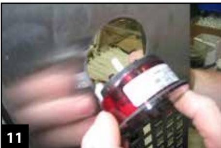
**STEP 16** - Pull thermometer and wires through the thermometer panel. (See image 11).
