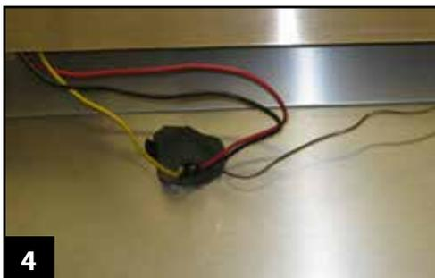
**STEP 4** - Remove perm gum from hole that is drilled through cabinet facing. Pull sensing bulb through hole. (See image 4).
