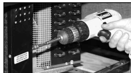
2 - Removing ballast box cover
