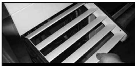
2 - Louvered grill hinges out then unhooks for removal
