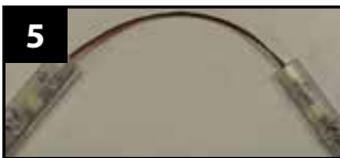
The units can be connected from either end. Do not exceed 6 total units per string.
