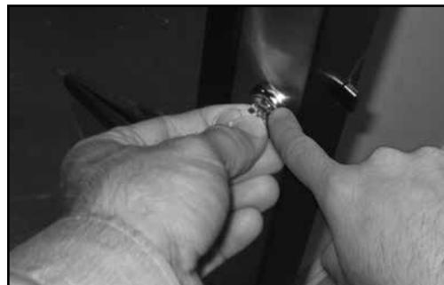
6 - Installing new plug / key receptacle
