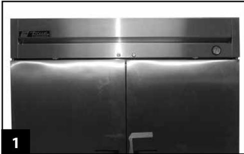
**STEP 1** - Remove the top, side, and bottom Phillips screw to the louver panel. (See image 1).
