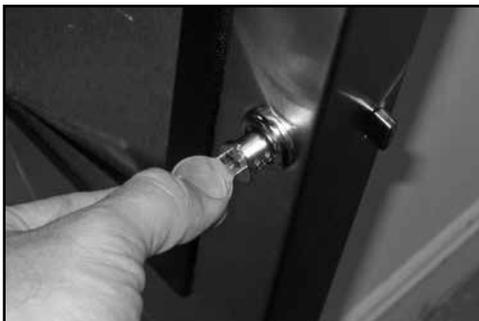
3 - Removing plug / key receptacle
