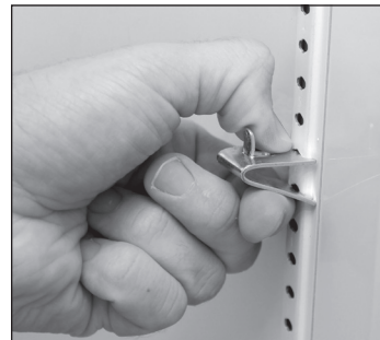
Fig. 12. You may need to squeeze or twist the bottom of the shelf clip to install.
