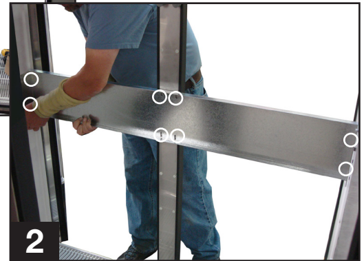
2 Bracket removal. Thumb screw locations.
