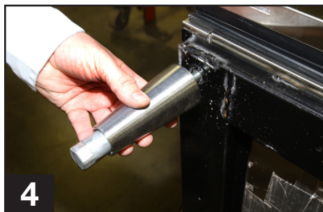
Thread leg into cabinet bottom frame rail.
