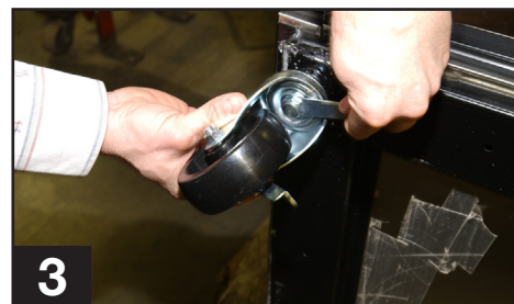
Use the tool provided to tighten the castor into place.
