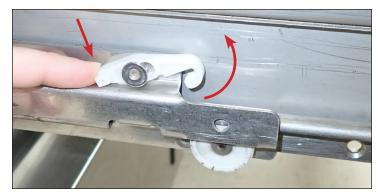
Fig. 2b. Push the back of the retainer down.
