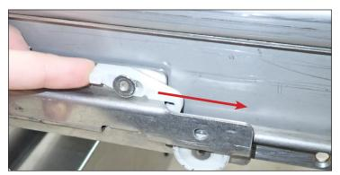
Fig. 2a. Push the retainer forward.
