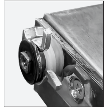
Fig. 7. Keep the washers in their original order.
