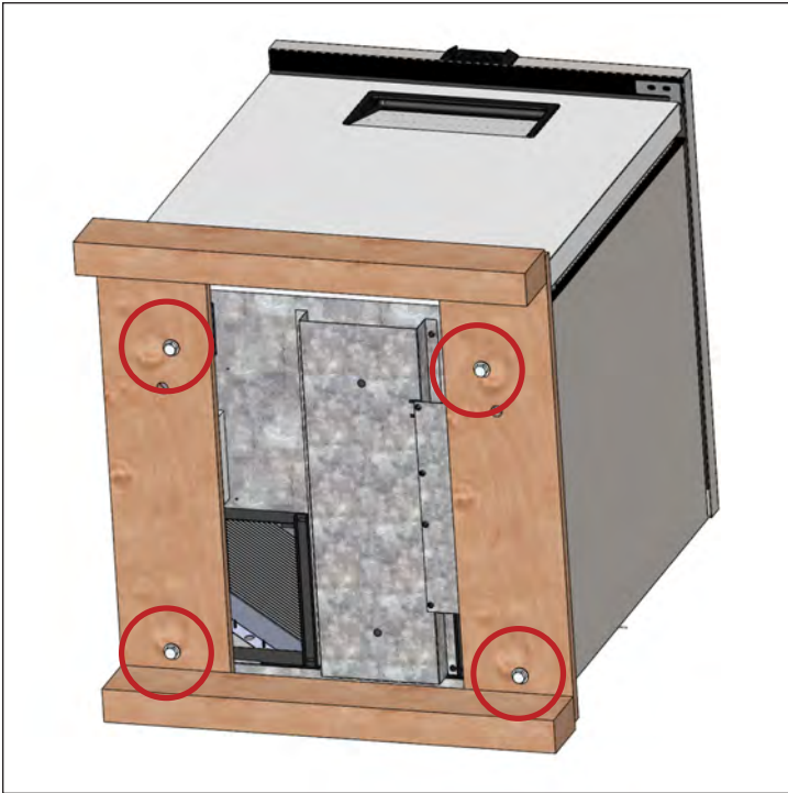
Fig. 3. Remove all shipping bolts.
