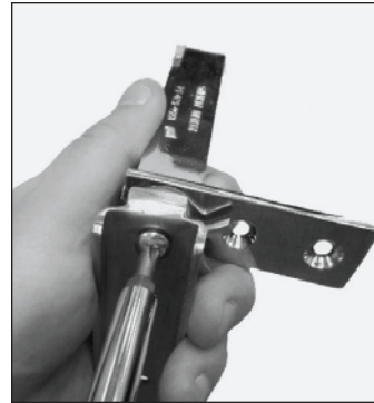
Fig. 6. Remove the hinge bracket from the cartridge spring and then rotate it.
