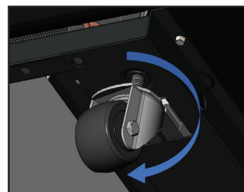
Fig. 6. Position multiple shims at 90° angles.
