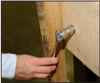
Removing skid from bottom of cabinet.
