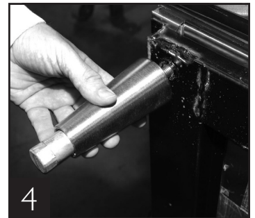
4 Thread leg into cabinet bottom frame rail.
