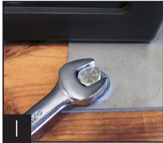
Removing bracket from skid.
