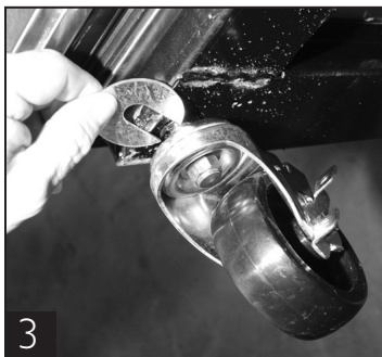
Use shims as necessary to level cabinet.
