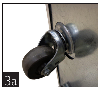
Installing castors (shims)
