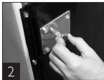
2 Reinstall leg levelers at bottom of cabinet.
