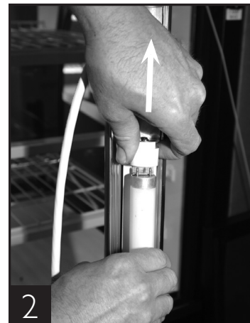
Remove bulb by gently pulling up on spring loaded lampholder.
