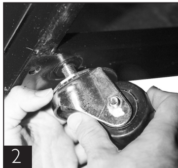
Thread castors into existing leg leveler holes.
