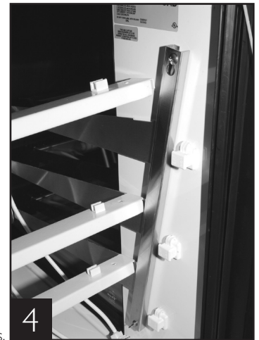
4 Install rear brackets.
