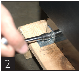
Removing bracket from cabinet.
