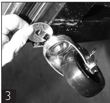
Use shims as necessary to level cabinet.
