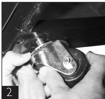
Thread castors into existing leg leveler holes.
