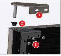
Fig. 7b. Top hinge component assembly.
