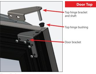
Fig. 4a. Top hinge components.
