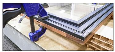
Fig. 6. Be sure the overlay's center slot is positioned at the top of the door.
