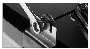
Fig. 1. Adjust the roller.
