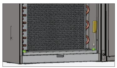
Fig. 5. Remove the condensing base bolts.
