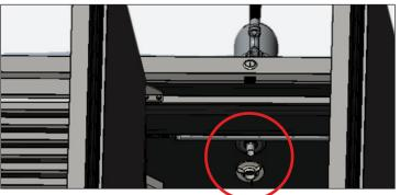
Fig. 1. Spill tray tube nut installation location.
