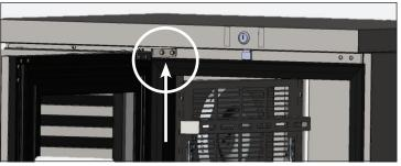
Fig. 1. Top hinge bolt locations.
