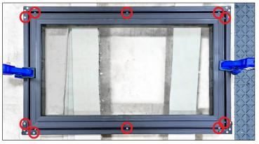
Fig. 7. Cabinet door predrilled hole locations.
