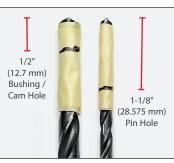
Fig. 8. Mark the hole depths on the drill bits.
