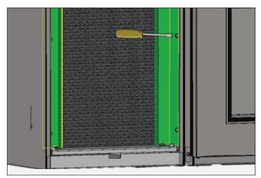
Fig. 6. Remove the coil brackets.
