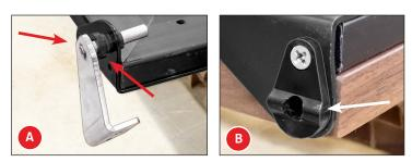
*Fig. 5.* Remove the top hinge pin & bushing (A) and the door cam riser (B) from the hinge brackets. Do not remove the hinge brackets.
