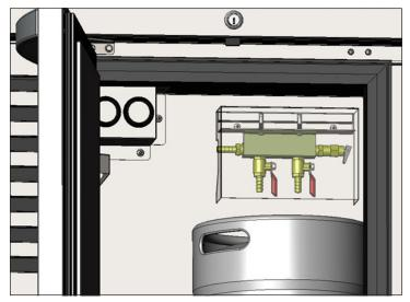
Fig. 2. The 2-way distributor manifold.
