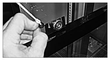
Fig. 6. Slide the the black tab holding the door cord out the back
