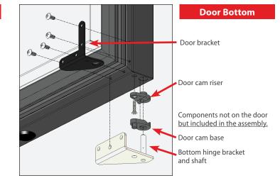
Fig. 4b. Bottom hinge components.
