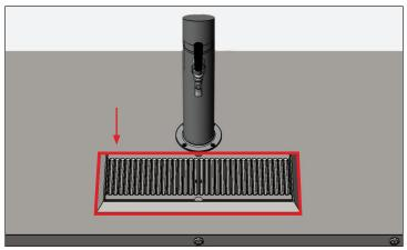
Fig. 4. Apply silicone around the spill tray.
