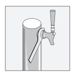
Fig. 1. Carefully remove the faucet.
