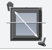
*Fig. 6.* The current bottom door bracket will be the new top door bracket.
