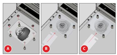
Fig. 6. Install castor shims in pairs.
