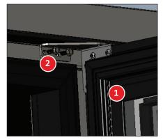
Fig. 10. Install the top hinge and the door.
