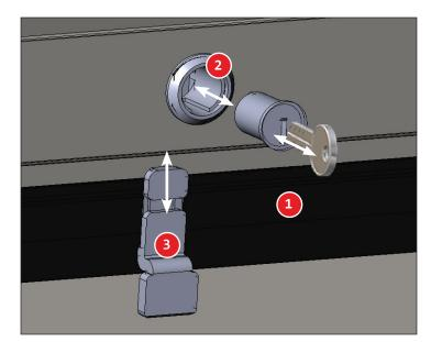
Fig. 1. Front view of removing/installing components.
