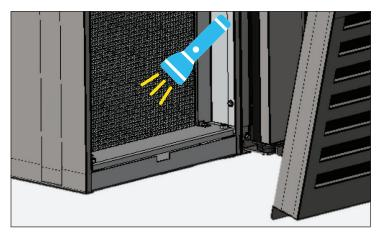
Fig. 4. Verify all blockages have been removed.
