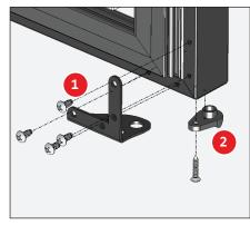
Fig. 7a. Bottom hinge component assembly.
