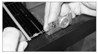
Fig. 5. Remove the door cord from the roller bracket.
