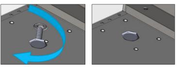
Fig. 1. Turn the leveling legs clockwise to lower the unit.
