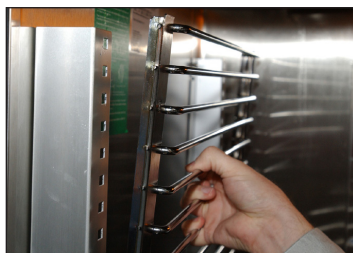
Fig. 7b. Installing kit #2 rod tray sides.
