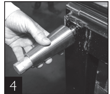
4 Thread leg into cabinet bottom frame rail.
